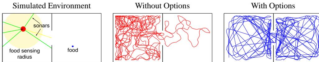
Figure 7: The simulated robotic foraging task. The picture on the left shows the five sonars, the doorway sensors, and the food sensor. The graphs on the right hand side represent the position of the robot during a random walk.
